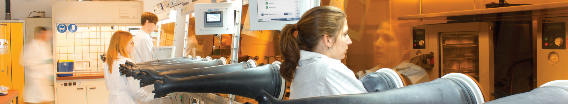
The Fraunhofer IZM's 10 m battery development and assembly line for the high-precision manufacturing of minute custom-design micro batteries
